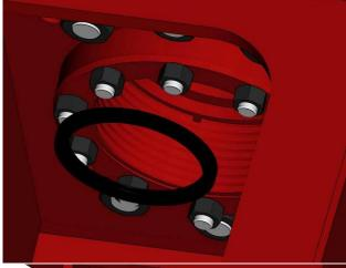
2 Insert the piston rod assembly into the liner and attach both to the inside of the retainer flange.
