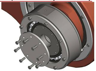
**4** Slide the main bearing and shims free of the crankshaft.
