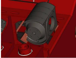
Unbolt and remove the main bearing cover.
