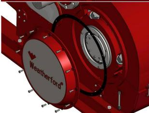
**3** Remove the back cover of the power frame.
