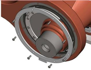
**7** Reinstall the main bearings as per 5.3.4.
