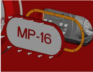
5 Unbolt the wrist pin retainer plate from the crosshead.
