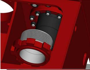
**5** Remove the liner and piston rod assembly from the power frame.
