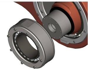
2 Unbolt and remove the outer bearing retainer from the crankshaft.
