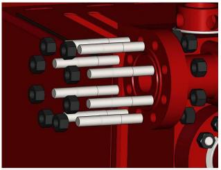
Unbolt the Discharge Pulsation dampener from the Discharge cross and carefully lift from the power frame.
