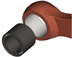
3 Heat the inner race of the wrist pin bearing and then slide into position on the wrist pin. Allow to cool before going any further with the assembly procedures.
