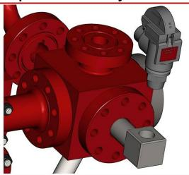
**4** Unbolt the discharge cross from its support and the discharge manifold, and remove.
