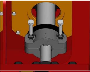
2 Rotate the pump so the crosshead extension is at the end of its suction stroke (fully retracted towards the power end).
