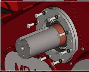
6 Use the jackscrew holes in the pinion bearing carrier and remove it and the spacer from the power frame.
