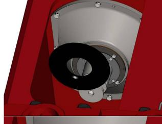
Remove the bolts affixing the wiper box to the diaphragm plate.
