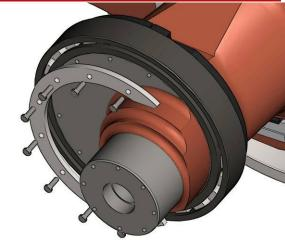
5 Slide the crankpin bearing inner race off of the crankshaft.
