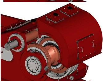
**5** Reattach the main bearing covers onto the power frame.
