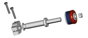
Re-install the piston, ensuring that the seal remains properly aligned with the groove in the piston hub. Lock into position using the piston rod nut, and torque to 1,000 ft. lbs. torque (on a 1.5" piston rod nut).
