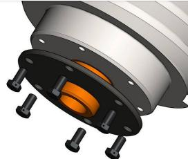
Remove and replace the upper valve stem guide, then replace and bolt the retainer plate into position.
