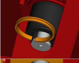
Rotate the pinion shaft bringing the extension rod and piston rod together and install the piston rod clamps.
