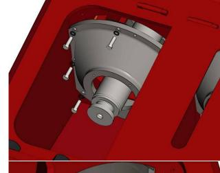
2 Rotate the pump so the crosshead extension rod is fully extended towards the fluid end. Unbolt the extension rod from the crosshead.
