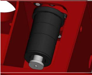
Remove the seal from the counter bore inside the liner retainer flange.
