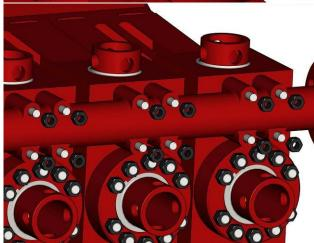
If maintenance is complete, reattach the piping to the suction manifold. Check that all components are properly installed and secure, then reengage pressure to the system.
