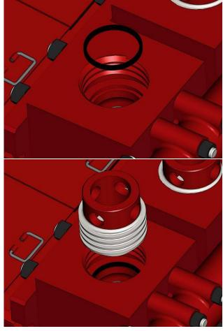
Coat the bottom seating surface and outside of the valve covers with grease and screw into place over the valve bores.
