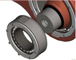
5 Install the inner retainer of the main bearing and bolt all retainers in accordance with the Torque Chart, page 53.
