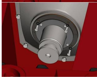
Slide the wiper box off the crosshead extension and out of the pump frame.
