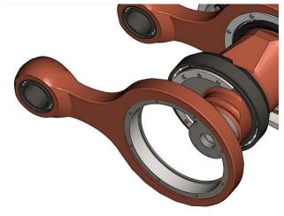
**2** Unbolt the main gear from the crankshaft.
