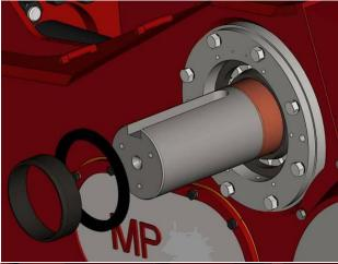
**5** Unscrew and remove the bolts and washers securing the pinion bearing carrier to the power frame.
