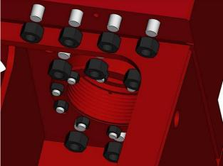
**3** Reinstall and bolt the retaining studs to secure the pump into position on the power frame.
