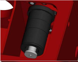
3 Slide the liner lock into place around the liner, and screw into the retainer flange of the fluid module.
