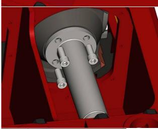
3 Carefully slide the extension rod free of the crosshead and remove.
