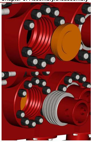
Once maintenance is complete and the pump is reassembled, run for approximately 15 minutes, then shut down the pump and release the pressure. Tighten the valve corner again with a sledgehammer and resume pumping.
