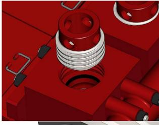
2 If replacing the valve stem guide, first unbolt and remove the retainer plate from the upper valve cover and remove.
