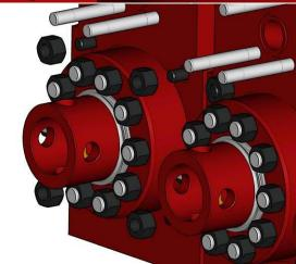
**3** Unbolt the inner retaining studs to free the fluid modules from the power frame.
