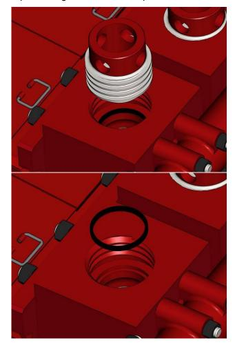
2 Remove the upper valve cover seal from the fluid bore.
