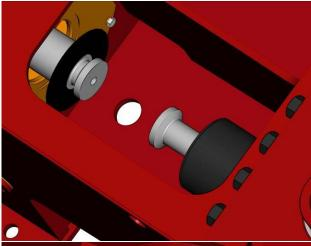
Remove the O-Ring from the split ring holding the liner lock in place, and slide the split ring free of the liner.
