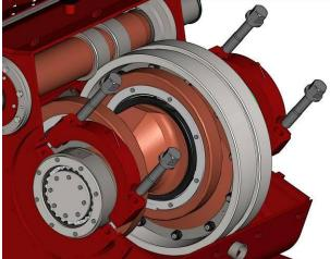
5 Slowly lift the crankshaft assembly free of the pump frame.
