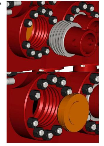
2 Remove the lower valve cover from the bore.
