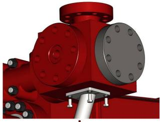
2 Reattach the Pressure Relief Valve, Pulsation Dampener and other components to the discharge cross.
