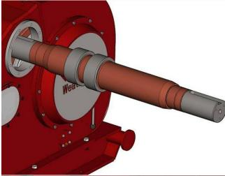
4 Slide the bearing carrier assemblies and gaskets over the pinion shaft and into the pump frame, exercising caution as they meet the inner race.
