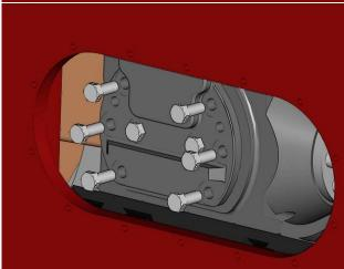
6 Utilize the tapped holes in the retainer plate to jack the wrist pin from the crosshead and mark to indicate which crosshead they were removed from.
