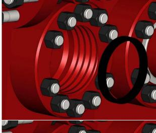
**4** Carefully remove the valve retainer from the valve bore.
