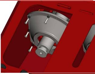
8 Check the wiper box for damaged or defective components, then reinsert into position on the diaphragm and bolt to secure.
