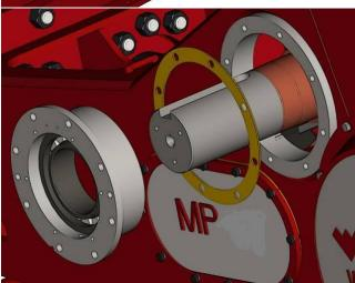
Install the pinion oil seal and race onto the pinion shaft.
