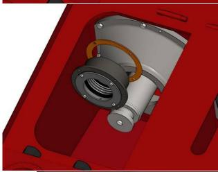
**9** Reinstall the baffle into position on the extension rod.
