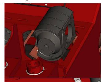
2 Remove the four (4) bolts which affix the crosshead guides to the frame.
