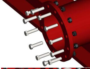
2 Remove the cap screws connecting the suction modules to the suction manifold.
