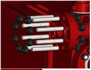
2 Remove the nuts connecting each of the discharge modules to the discharge manifold.
