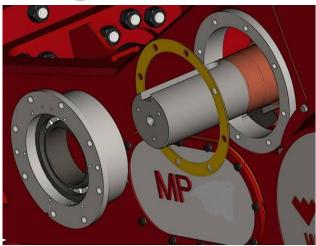
9 Slide the shaft out of the pump frame. Since the bearings are carrier mounted, the shaft can be removed out of either side of the frame. However, be sure to note its original orientation, as it should be replaced facing the same direction.
