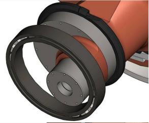
4 Install the inner retainer to lock the bearing into place.
