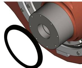
Install the main bearings into the bearing carriers. Secure using the outer retainer ring.
