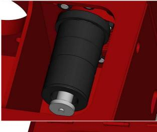
**2** Mark the outer surfaces of the wiper box and diaphragm plates to indicate their orientation in the pump frame.
