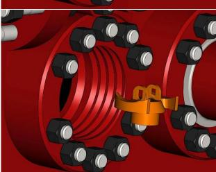
Slide the valve cage out of the fluid bore, exercising care not to hit or damage the valves.
